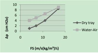
Fig. 5. Pressure drop for the centrifugal tray
