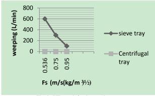
Fig. 3. CFD result for the weeping rate
