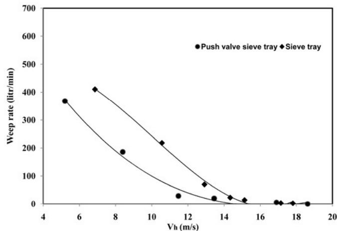
**Figure 6.** Weeping rate of sieve and push valve sieve tray at liquid rate of 45 m<sup>3</sup>/mh
