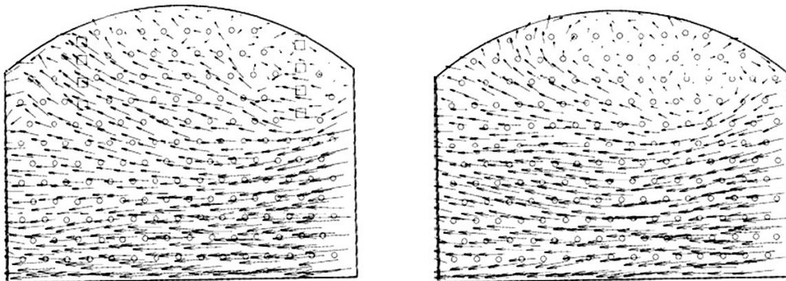
**Figure 3.** : Liquid velocity vectors at 38 mm above the tray deck,  $Q_L = 17.8 \times 10^{-3} m^3 / s$ ,  $F_s = 0.801 m/s(kg/m^3)^{0.5}$
