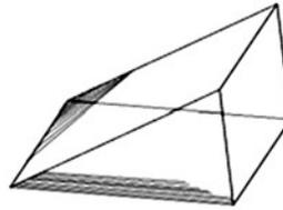
**Figure 1.** Simulated Push valve on the sieve tray
