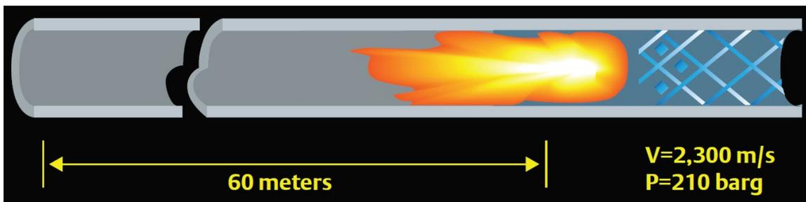
*Figure 9: Overdriven (Unstable) Detonation*
