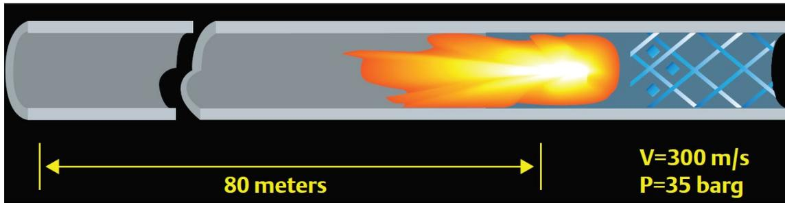
**Figure 10: Stable Detonation**
